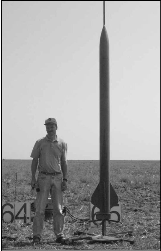
Photo Credit: Lance Lickteig Steve Klausmeyer's GO! Rocket - Level 3 certification project is ready to fly on an M1297.
